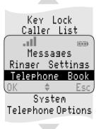
Selection lists (e.g. telephone book) and the features menu are shown in the display as a three-line excerpt. Using the arrow key, the lines of text can be scrolled up or down. A selectable entry is shown inversely, with a dark background.
